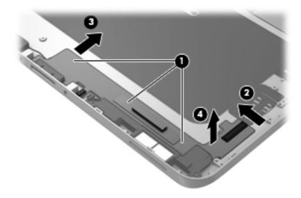
Reverse this procedure to install the docking connector cable.
